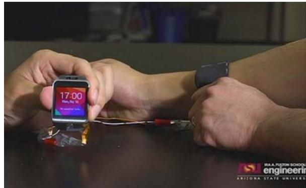
Inventors have created lithium-ion batteries that can stretch to more than 150 percent of their original size, while remaining capable of powering devices.
