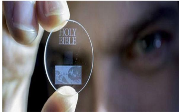
dimensions are the size and orientation of the dot. The nanostructures created by the technology can be read using an optical microscope in tandem with a polariser (a filter designed to block specific polarisations of light).
